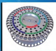
39 quartz cuvettes in water bath 37°C
